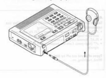
Use the HP/SPK VOLUME knob to control the volume of the headphones. The sound from the internal speaker is muted automatically when headphones are connected.
